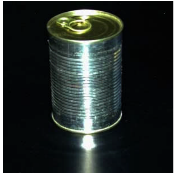
This steel can is coated with tin for corrosion protection
