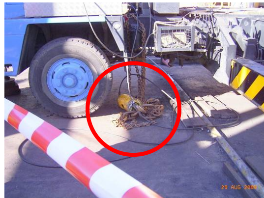
The final location of the auxiliary hook after uncontrolled free fall into the working environment.
