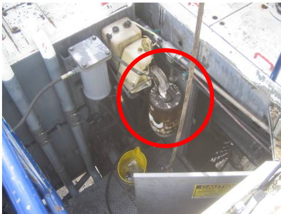
The final location of the auxiliary hook after an uncontrolled free fall into the working environment.
