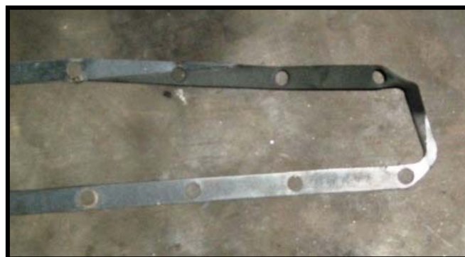
The intake gasket of the diesel engine system.
