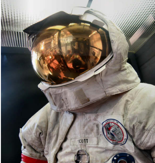
A space suit from the Apollo 15 mission to the moon, note the visor's gold coating to protect the astronaut from the infrared radiation from the sun.
