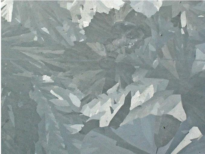
A close up of the surface of steel that has been galvanised with zinc. This crystalline coating is what protects steel from rusting.
