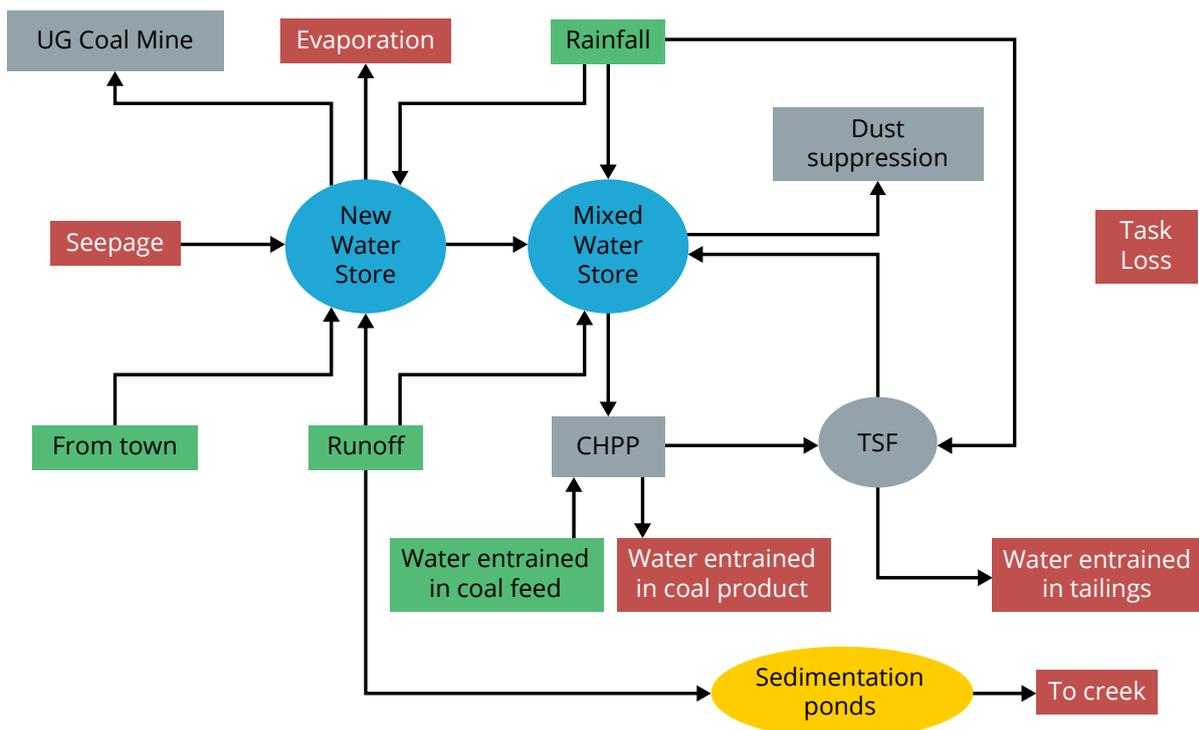
The flowmeter monitoring the transfer of makeup water from the new water store to the mixed water store failed during the year and had to be replaced. An estimate of the water transferred was made by utilising available reporting data to determine an average requirement (25 ML/month) for the accounting period (300 ML/year). Water used in Dust suppression was estimated using truck counts and expected water volume per truck (648 ML). The estimates were considered to be of low confidence.
